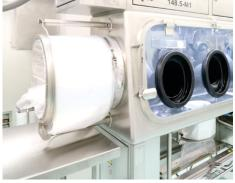
In cooperation with a customer we develop an isolator regarding the process requirements (sampling, weighing, dispensing, sterility testing...). Dimension, shape, number of gloves, additional equipment, and atmosphere are adjusted to planned work and are finally determined on a real size steel MOCK UP model. With our experience we can offer the most suitable equipment solution for our costumers' needs.
