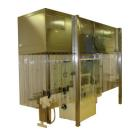
Product protection ISO 4 to ISO 8 (ISO 14644-1:1999) Class A to D according to GMP
