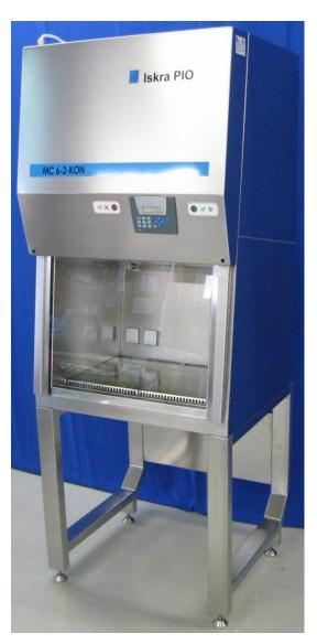
Microbiological safety cabinet executed in protective **class II** according to EN 12469:2000 and DIN 12980:2005 assure ISO 5 (ISO 14644-1:1999), class A (GMP) clean conditions inside working area. Clean conditions are assured by H14 (EN 1822) HEPA filtration of recirculating and exhaust air. Laminar vertical air flow in working area and air curtain on the front aperture assure controlled clean conditions in the chamber and prevents material leakage from the chamber.
